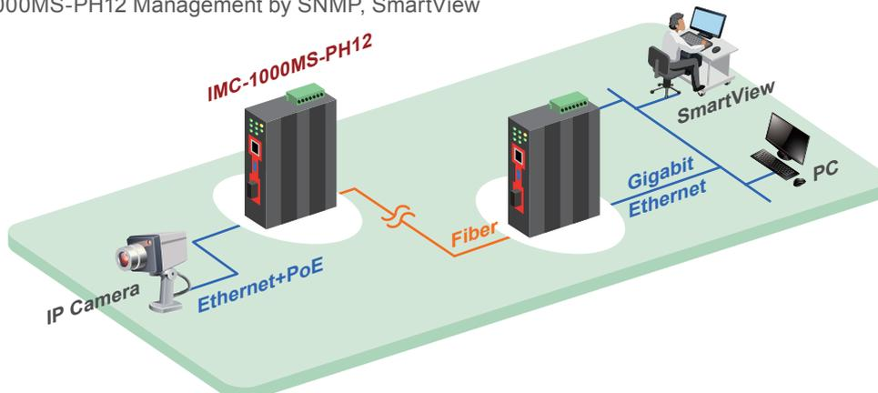
Figure 2 : IMC-1000MS-PH12 Application in Remote, In-Band Management
