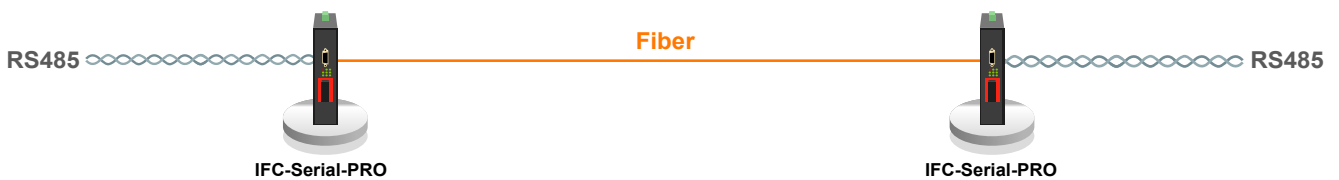
Figure 7 : Fiber Point to Point topology & application
