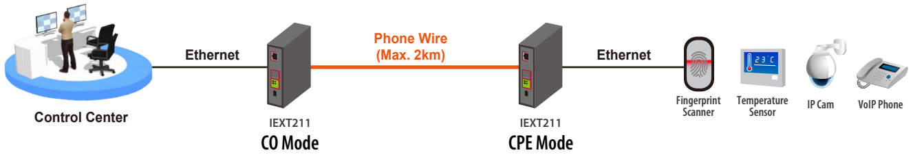
Figure 1 : Distance extend for Ethernet Application
