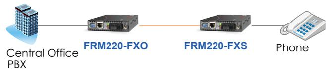
Figure 3 : Selectable FXO or FXS mode
