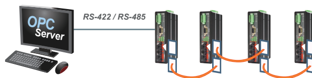
Figure 4 : RS-422/485 Fiber Daisy Chain
